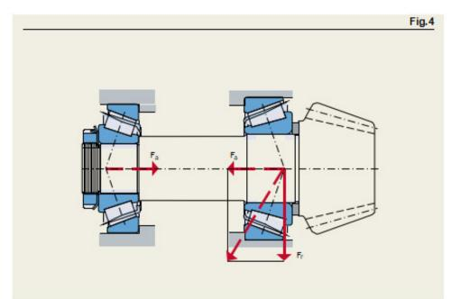
When determining preload, the preload force required to provide an optimum com- bination of stiffness, bearing life span and operational reliability should be calculated irst. Then calculate the preload force to be used when adjusting the bearings during mounting; the bearings should be at ambient temperature and should not be subjected to any other load.
